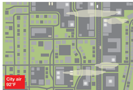
Left: Without white roofs. Right: With white roofs. Pavements and roofs comprise about 60% of city surfaces. White roofs and cool pavements can help reflect away the sweltering temperatures of summer urban heat islands, improving air quality and comfort.
